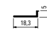
650 101 Edge protection 567 257.17 Push-in gasket Material: Plastic Surface finish: Silver PU: 100 running metres
