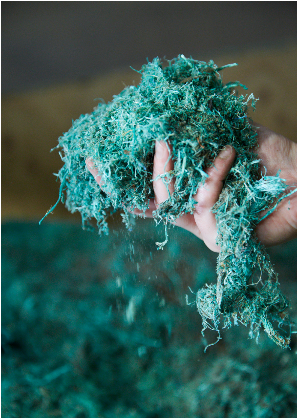
The discarded and obsolete fishing gear, ropes etc. are cleaned before being made into granulates.
